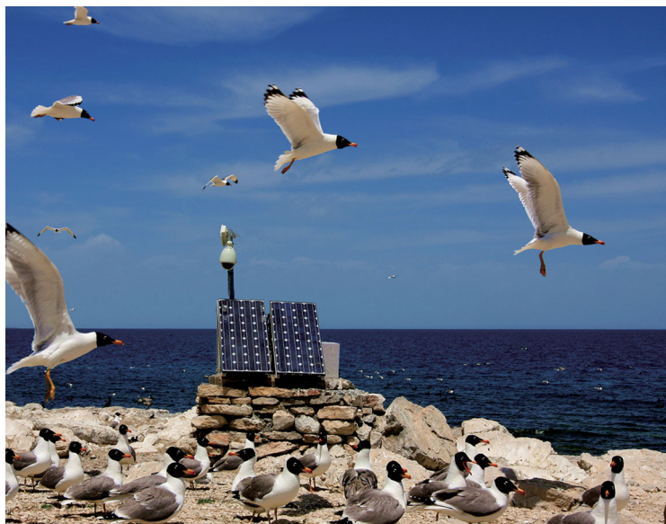
Figure 7. A video monitoring system deployed in the core protection area of the Qinghai Lake nature reserve, networked to the CNGrid backend.
